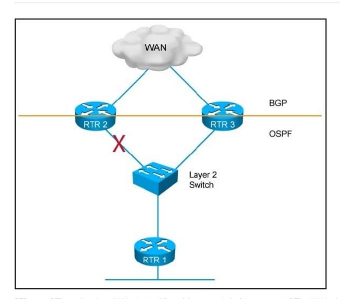
RTR 1 uses RTR 2 as the primary WAN exit point. When a failure occurs in the link connected to RTR 2 LAN, it takes about 40 seconds for RTR 1 to use the backup path via RTR 3.
