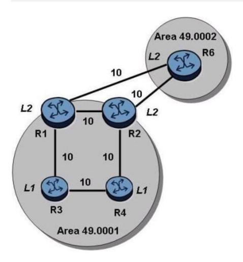
Examine the physical topology of the IS-IS network, the metrics of the links and the levels of the routers. All routers have a system address included in IS-IS. Which of the following describes the route that router R4 will use to reach the system address of router R6?
