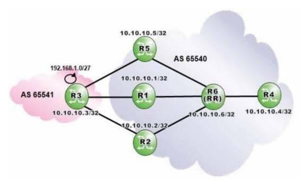
Router R6 is a route reflector with clients R1, R2, R4 and R5. Router R4 receives three routes from router R6 and is configured with ECMP 3. Given the following BGP configuration on routerR4, how many primary and backup paths will be present in router R4\\'s BGP routing table?
