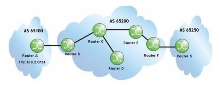
Routers C and E are route reflectors. When the update for prefix 192.168.2.0/24 is received at router F, what will be the Originator\_ID attribute?
