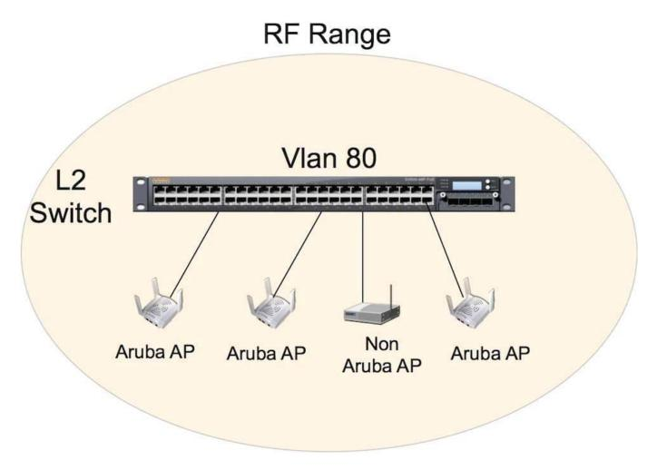
Referring to the diagram provided for this question, an employee brought an unauthorized AP from home and attached the LAN port to the cubicle Ethernet port. All Aruba APs and AMs as well as the employee AP are in VLAN 80 and within RF range of each other. No traffic from the wired or wireless network has passed through the unauthorized AP yet, but the AP began wireless broadcasts. How will the Aruba system initially classify the employee\\'s non-Aruba AP?
