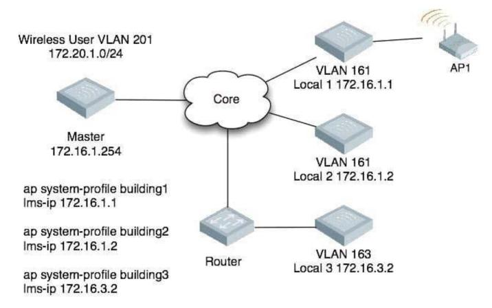
The above diagram has one master and three local controllers. AP1 GRE terminates on controller Local 1.
