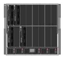
As shown in the exhibit, four BL460c G6 Server Blades are installed in a c7000 enclosure. What is the maximum number of BL680 Server Blades that can be added to this enclosure without powering off any blade?
