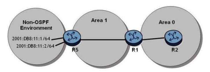
The route table on router R2 shows the system address of router R5 but it does not show any of the interfaces from the non-OSPF area.
