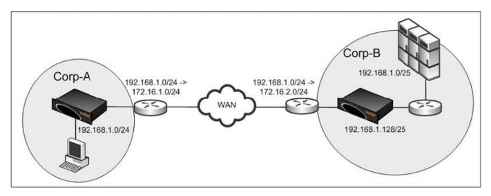
Corp-A and Corp-B have overlapping address space and therefore the network administrator implemented NAT to overcome this. Users from Corp-A NAT to 172.16.1.0/24 and users from Corp-B NAT to 172.16.2.0/24. Users in Corp-A use the destination address of 172.16.2.0/24 to access the resources in Corp-B. The servers in Corp-B use the client IP for authentication. What do you need to do in order to make this deployment work? (Select 2)
