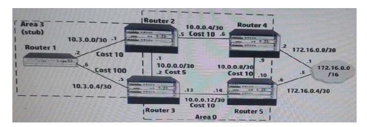
Router 4, which is an HP Comware router, redistributes Routing Information Protocol (RIP) routes into Open Shortest Path First (OSPF) process 1. Router 4 has several dozen IP routes, and the network administrator wants to minimize the number of external routes throughout the entire OSPF AS. How can the administrator meet this requirement?
