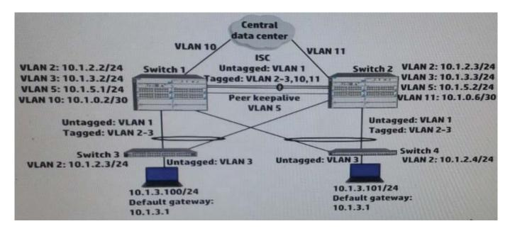
Switch 1 and switch 2 run open Shortest Path First (OSPF) on all VLANs. Both switches establish an OSPF adjacency to a router at the main data center. Exhibit shows shoes some virtual Routing Redundancy Protocol (VRRP) and OSPF settings on Switch 1 during normal operation.
