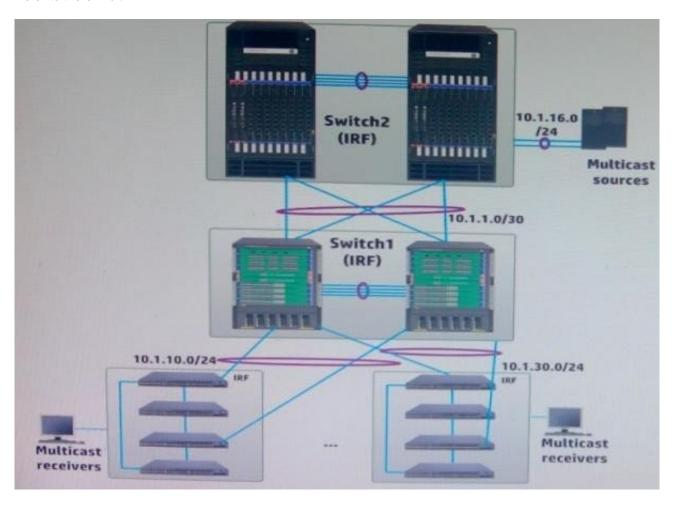
All connections between switches are 10 Gbps. Switch is an Intelligent Resilient Framework (IRF) group with two member. Switch2 is an IRF group with two members.
