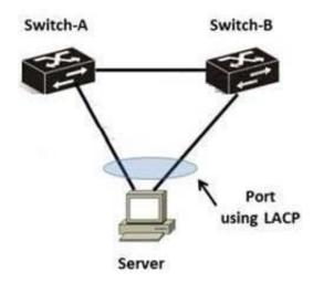
A network administrator has a server with a single link to the network. The company is concerned about redundancy and wants to implement a solution like that shown in the right-hand side of the diagram.
