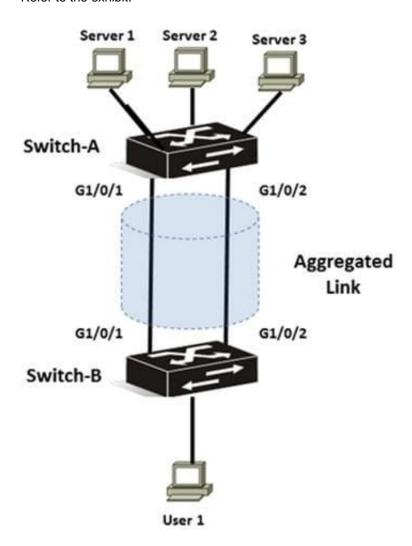
A network administrator needs to configure link aggregation using static LACP on Switch-A, which is an HP Comware switch. Which configuration accomplishes this goal?
