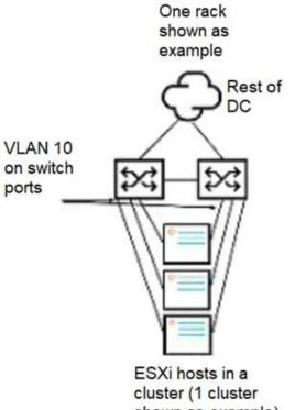
NSX settings Logical switches: VNIs 5000-5100 VXLAN transport settings: VLAN ID: 10 NIC teaming: single active adapter = LACP lag Control plane mode: Unicast
