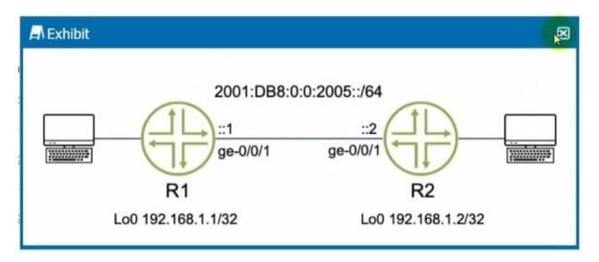
You are asked to configure OSPF between routers R1 and R2 using IPv6 addresses. Which two tasks will accomplish your objective? (Choose two.)
