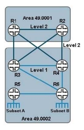
R5 must advertise Subnet A into IS-IS so that Subnet A and Subnet B can communicate. Subnet B must be able to forward traffic to Subnet A and towards Area 49.0001. However, R5 should not be able to route traffic from Subnet A to Area 49.0001.
