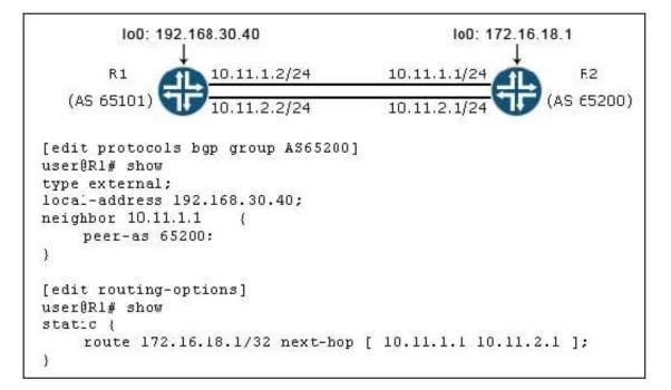
Referring to the exhibit, what must be added to the existing configuration to ensure that per-prefix load balancing occurs?
