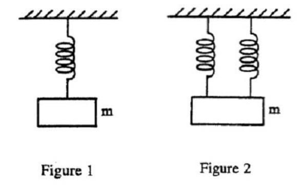
The mass in the first experiment is pulled down a distance A from its equilibrium position and then released from rest. The mass will then oscillate with simple harmonic motion. As the mass moves up and down, energy is dissipated due to factors such as air resistance and internal heating of the spring. The mass will no longer oscillate when the total energy dissipated equals:
