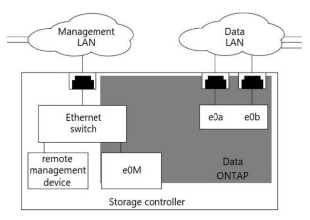
You are installing a new FAS cluster. The management network must be on tagged VLAN 11 for remote administration by a service provider. Referring to the exhibit, which two ports will allow service provider access to both cluster and node management LIFs? (Choose two.)
